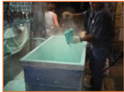
45' long, 600°F, powder coating line; semi-automated for fluidized bed coating
