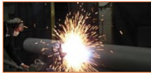
Metalizing capabilities up to 20' length parts
