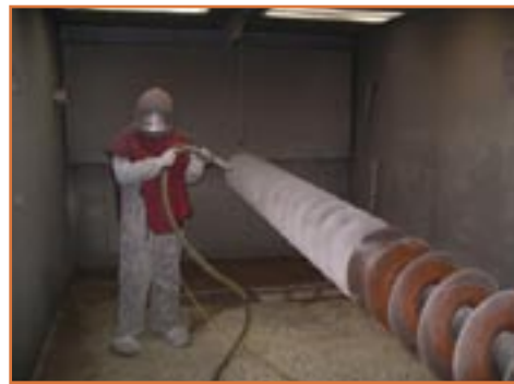
Abrasive blasting with six wheel conveyORIZED automated blast machine and 24' walk-in blast room as well as small blasting chambers
