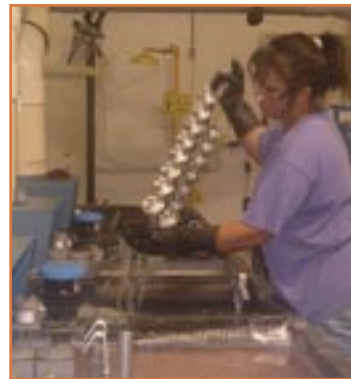
Complete high performance plating operation including a 13 stage, manual rack, hard coat anodize line and an 18 stage Diamonite hard plating line
