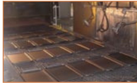
6' wide, 65' long, 850°F, conveyORIZED belt oven with fully automated reciprocating spray units
