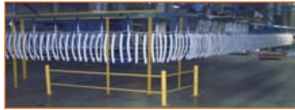
Automated 220' wet coating line with gas IR oven for plastics and other low temp curing products
